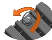
D) After unlocking, hold the ring of the screw and lift the top cover up slightly and pull it away from the wall in the indicated direction.
